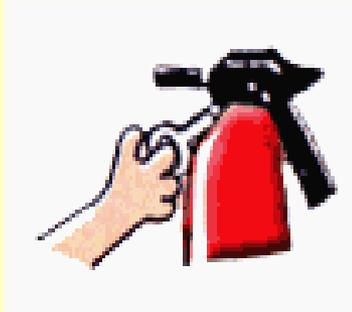
**5** **PULL**... the pin. Some extinguishers require releasing a lock latch, pressing a puncture lever or other motion.
